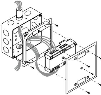
**Electronic Addressing** - The loop controller electronically addresses each module saving valuable time during system commissioning. Setting complicated switches or dials is not required. Each module has its own unique serial number stored in its on-board memory. The loop controller identifies each device on the loop and assigns a "soft" address to each serial number. If desired, the modules can be addressed using a laptop computer. No addressing switches are used.
